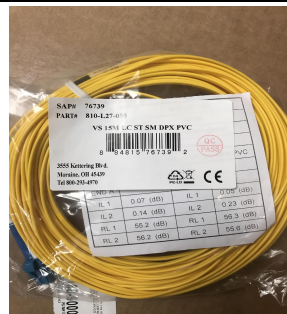
Figure 2: Fiber patch cable
